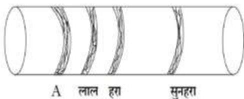
In given diagram value of carbon resistor is  $22 \times 10^5 \Omega \pm 5\%$ . Write colour of first ring A.
