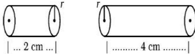
In the figure, resistivities of two conductors of same material are  $\rho_1 \Omega \cdot m$  and  $\rho_2 \Omega \cdot m$  respectively. Write the value of ratio of  $\rho_1$  and  $\rho_2$
